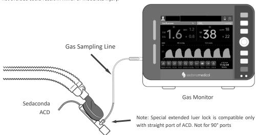
**DEVICE DESCRIPTION**: Gas Sampling Line. The medical device is non-sterile, disposable, single-use gas sampling line that enables sampling of respiratory gases. The gas sampling line is available in different end connection adapters to connect to monitors.
