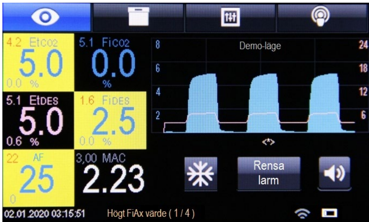
Figur 1.11 – Skärmen "Monitoring" (standardskärm utan FiCO 2 , FiAx)
